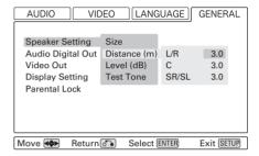
The L/R setting changes the distance of all speakers together. Pressing the up button adds 0.1m to each value, and pressing the down button subtracts 0.1m from each value.
